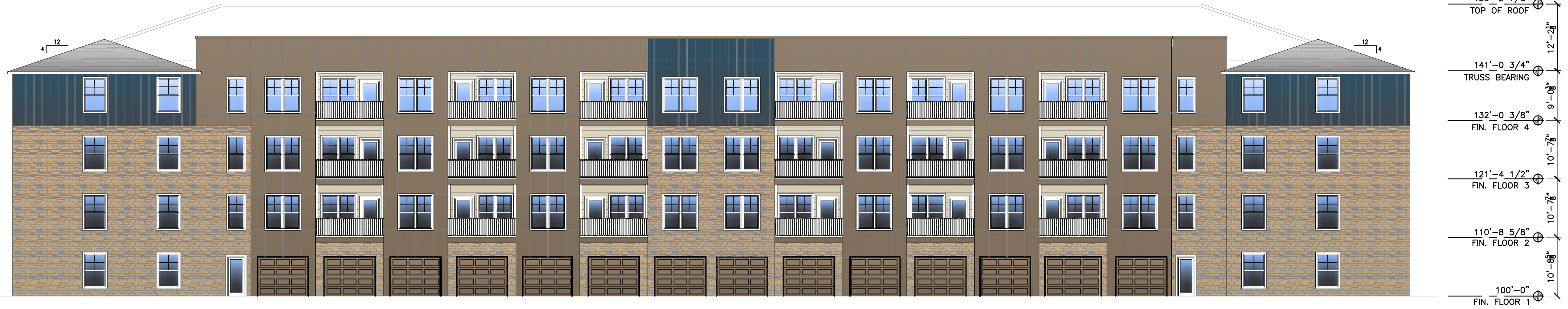
BUILDING TYPE 2 REAR ELEVATION 3/32"=1' 10'-8" 16' 1:128
