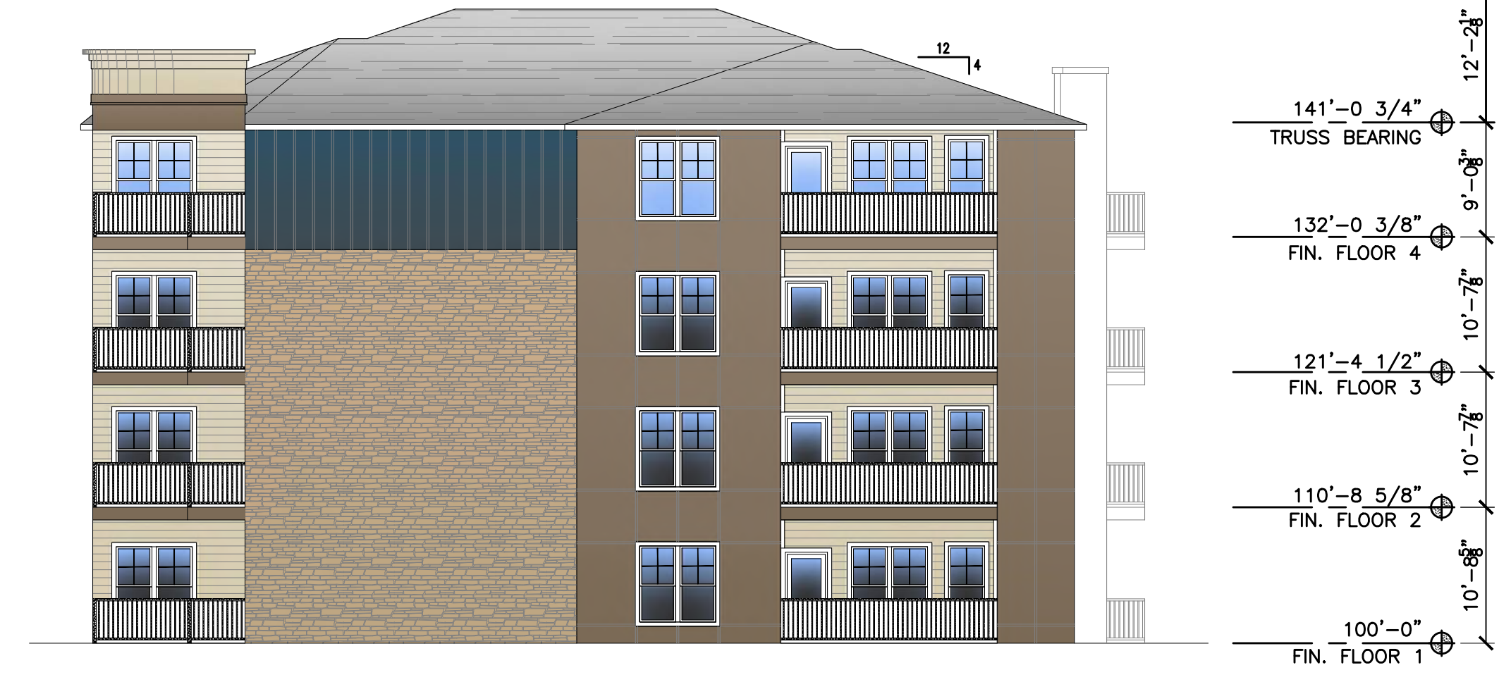
BUILDING TYPE 2 SIDE ELEVATION 3/32"=1' 10'-8" 16' 1:128
